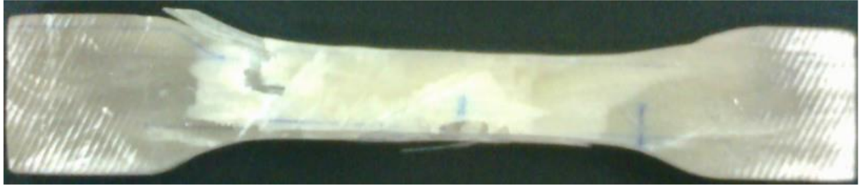
Figure 2 Tensile test specimen before testing
