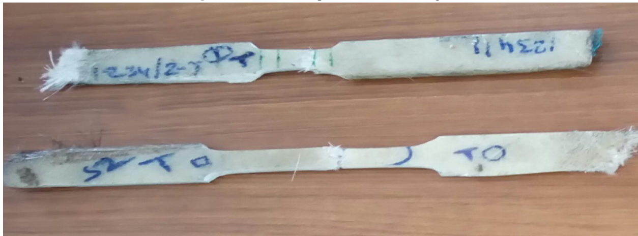
Figure 3 Tensile test specimen after testing
