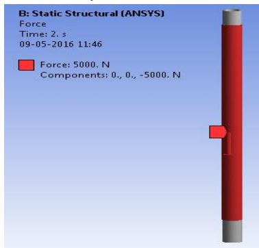
Fig.No.16. force applied on vertical beam 5000N
