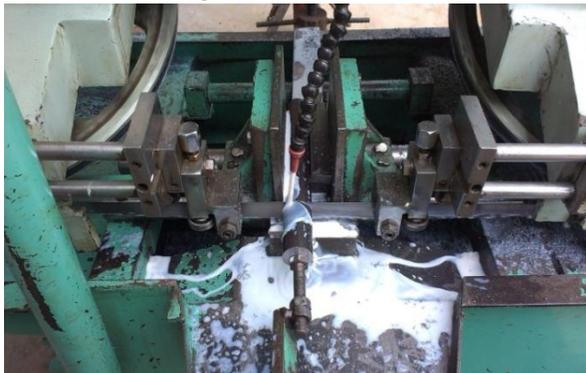
**Fig: 4.6** Cutting of workpieces on power hacksaw
