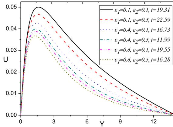
Fig. 2. (a) Velocity profiles at  $X=1$ .
