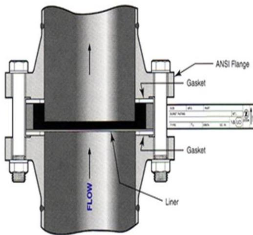
Fig4: Installed rupture disc[13]
