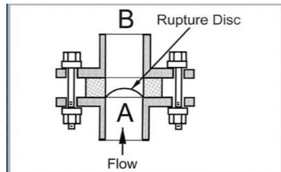
Fig 2: Rupture disk working principle [11]
