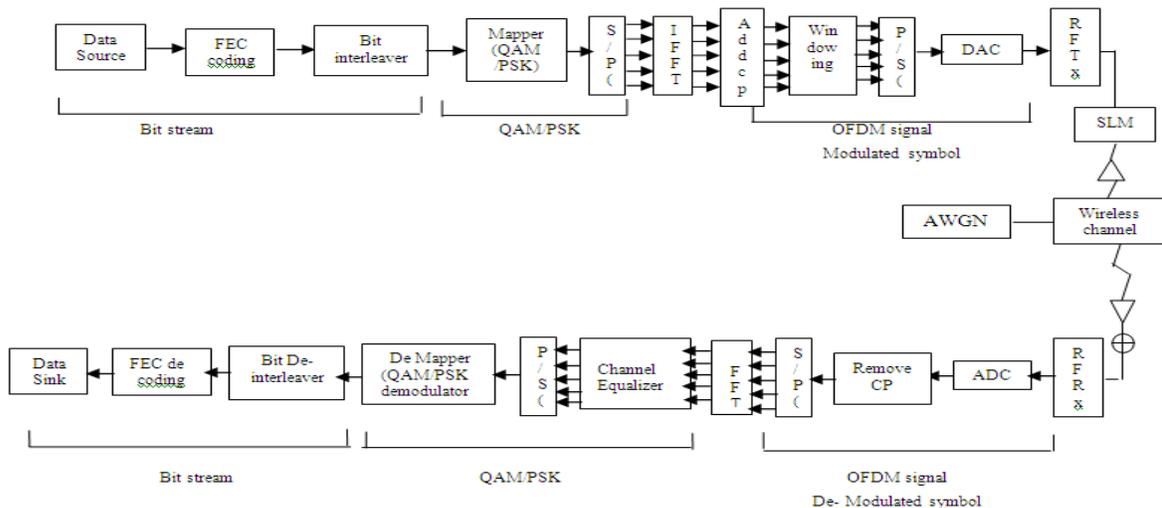
Figure 3 Transceiver of OFDM
