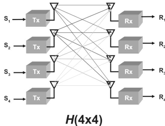
**Figure 4** Block diagram of MIMO system (4 \* 4)
