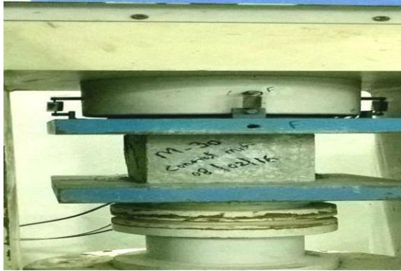
Fig 3: Compressive strength test
