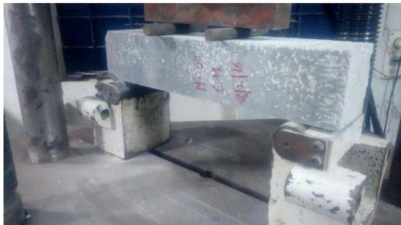
Fig 4: Flexural strength test
