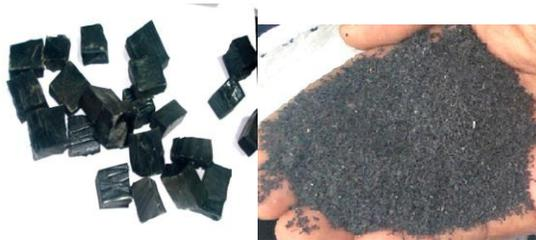
Fig 1: Crumb rubber fragments and powder
