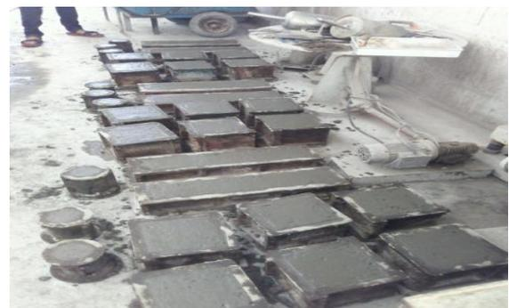
Fig 2: Specimen casting
