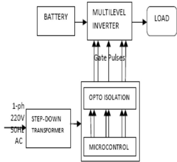
Fig 1: Block diagram of complete proposed system
