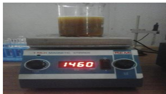
Fig 2: magnetic asscillator for mixing of nano particles with lubricant
