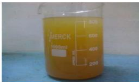
Fig 3: After Mixing of Nano particles in lubricant oil(PAG oil)
