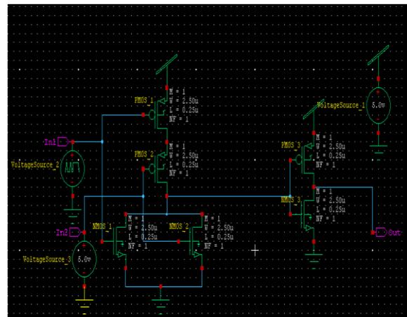
TRANSISTOR LEVEL CIRCUIT FOR OR GATE IN GDITECHNIQUE
