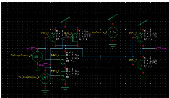
TRANSISTOR LEVEL CIRCUIT FOR AND GATE INGDI:
