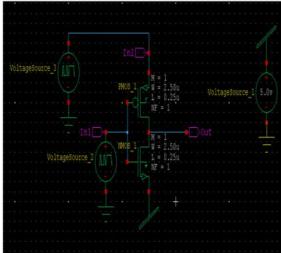
TRANSISTOR LEVEL CIRCUIT FOR XOR GATE IN CMOS TECHNOLOGY
