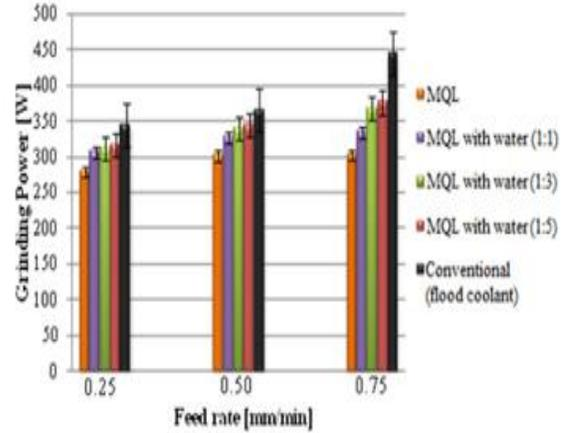
Figure 8. Grinding power results for each cooling-lubrication condition.
