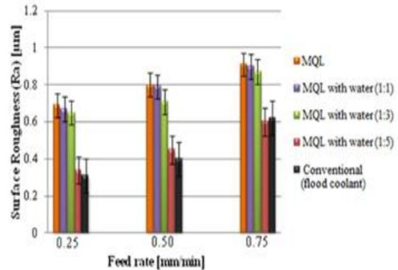
Figure 4. Surface roughness results for each cooling-lubrication condition.
