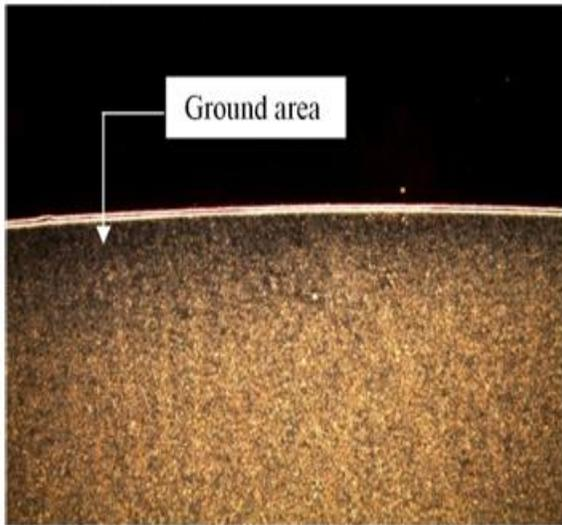
Figure 9. Optical microscopy for the traditional MQL condition (10x magnification).
