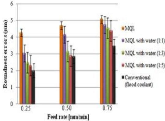
Figure 6. Roundness errors results for each cooling-lubrication condition.
