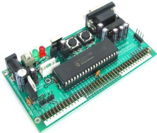
Fig.5 PIC Micro Controller
