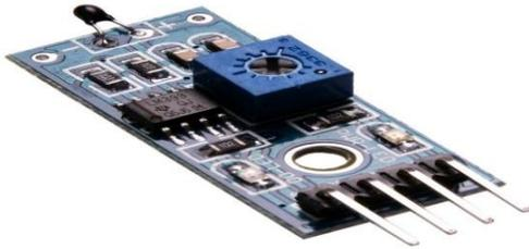
Fig.2 Temperature sensor
