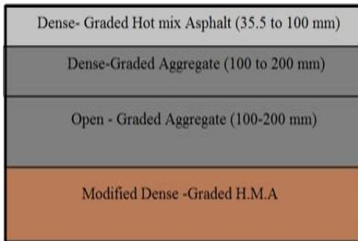
**TYPICAL LAYERS OF A FLEXIBLE PAVEMENT**
