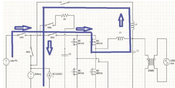
Figure 4. PV to Battery Charging
