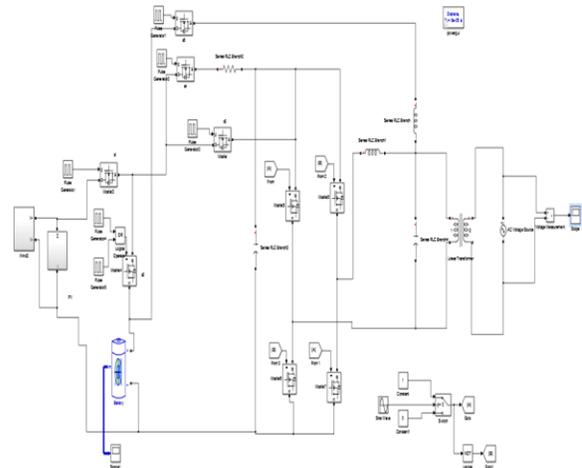
Figure 6. Simulation of Single Phase Inverter
