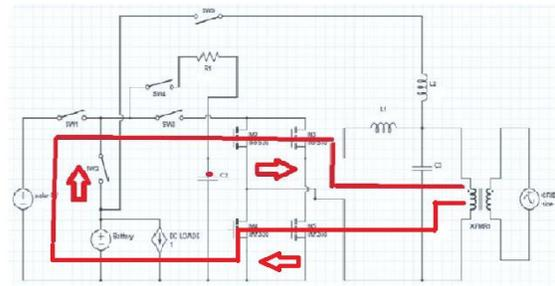
Figure 2. PV to Grid
