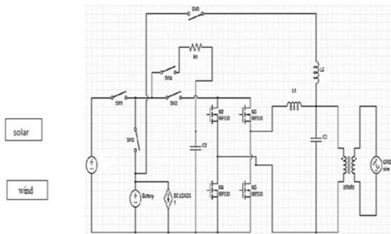
Figure 1. Circuit diagram of single phase inverter
