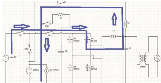
Figure 4. PV to Battery Charging
