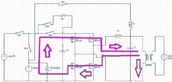
Figure 5. Battery to Grid
