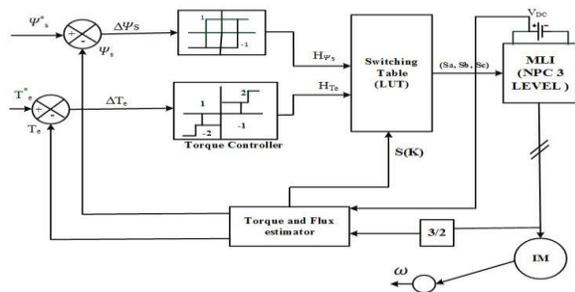
Figure 6: Block diagram of 3 level DTC technique
