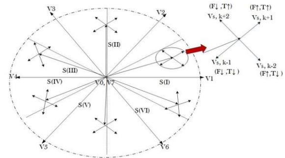
Figure 3: Selection of voltage vectors at changes in flux and torque [5]
