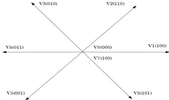
Figure 5: Voltage vector for two level inverter
