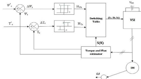
Figure 2: Block diagram of two level-VSI fed DTC
