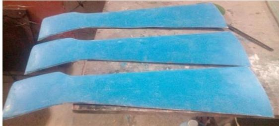
CFD analysis is conducted using FLUENT and the fabricated model is subjected to experimental analysis by mounting the blade to the ceiling fan hub.
