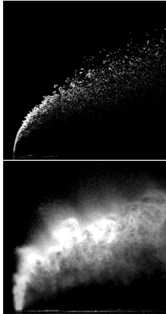
Fig:- Instantaneous images of liquid jet and spray in crossflow for same crossflow velocity and liquid flow rate. (Arrow shows the direction of air stream flow.) [7]
