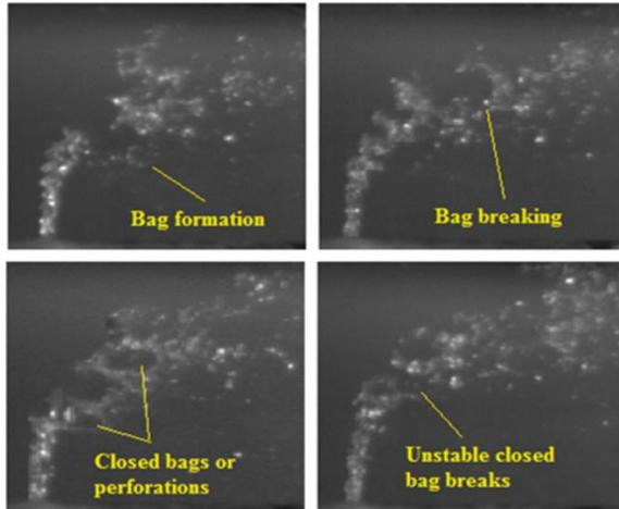
Fig:- Temporal images of q521 for 15 deg vane showing bag breakup mode.[11]
