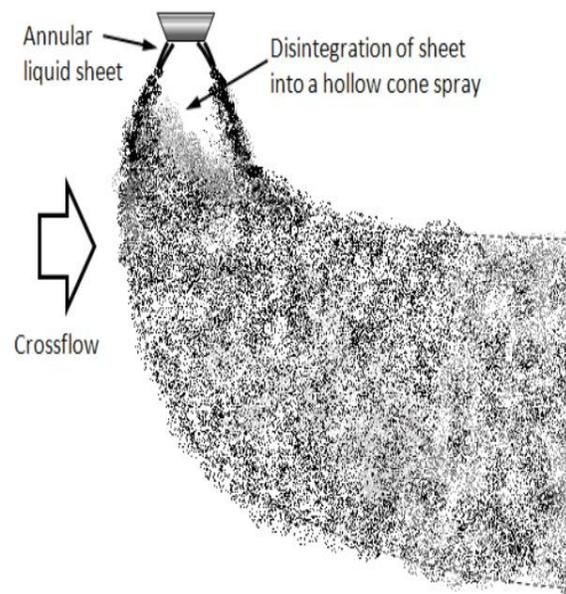
Fig:- Hollow cone spray in crossflow (adopted from [5]).
