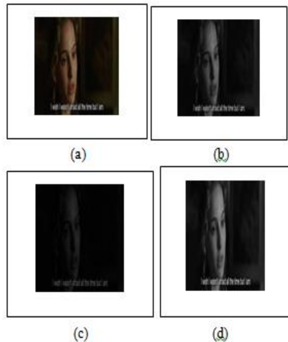
Fig.1 Preprocessing (a).Input image (b).Y image (c).U image (d).V image
