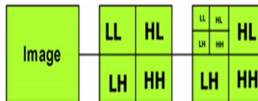
Figure 6.2 Decomposition of Image using DWT Discrete Wavelet Transform based steganography approach was proposed by Ahmed A. Abdelwahab et al. In this approach, the cover image is decomposed into four sub-images such as approximation coefficients (CA), horizontal detail coefficients (CH), vertical detail coefficients (CV) and diagonal detail coefficients (CD). Similarly, the secret image is decomposed into four sub-images. These sub-images are divided into non-overlapping blocks. The blocks of approximation coefficients of cover image are subtracted from approximation coefficient of secret image. The differences of these coefficients are called error blocks. The replacement of an error block is being done with the best matched CH block. Besides using CH block, we have done experimentation using CV and CD blocks also to see the effect on PSNR of the stegano image using the algorithm as proposed by
