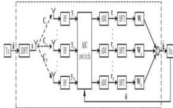
Fig.1. Illustration of the mixed-ADC architecture for frequency-selective SIMO channels
