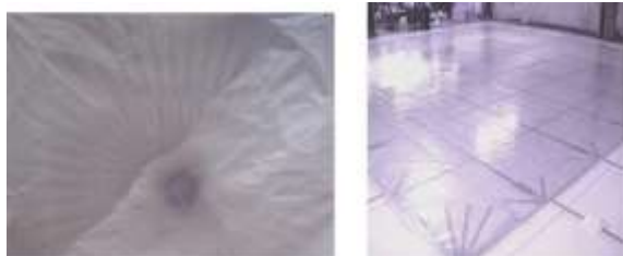
Figure 3. (Left) 3D 360° Radial Reinforced Panel & (Right) Large 40ft x 40ft Integrated Structure Panel for Decelerator Applications
