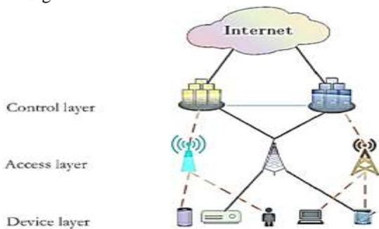
Fig. 1: The architecture of the D2D-supporting IoT system for smart cities.
