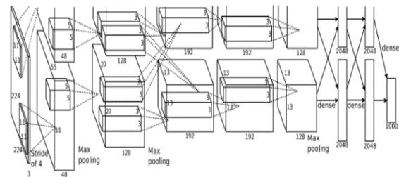
Figure 4: AlexNet Architecture
