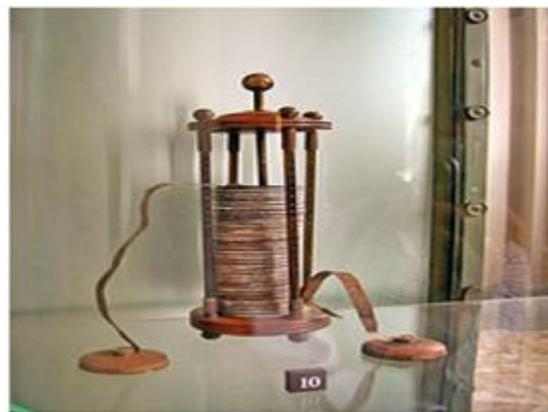
A voltaic pile, the first chemical battery
