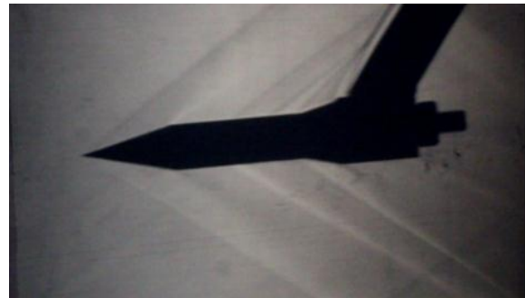
Fig.3 Testing of 90 degree wing in the supersonic wind tunnel
