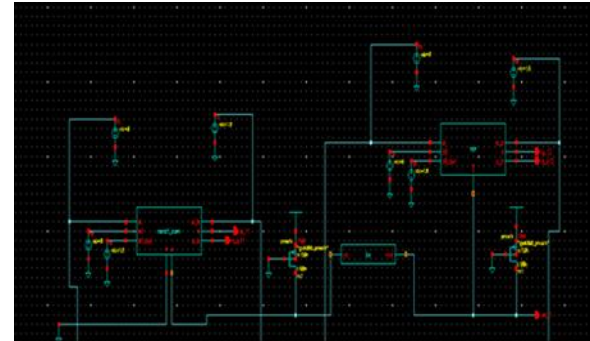
Fig. 14: Schematic for implementation of single bit line NAND-NOR type binary CAM cell
