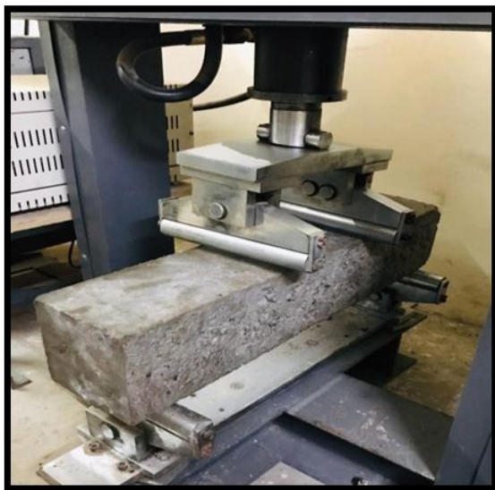
Figure 4. Placing of Beam for Testing
