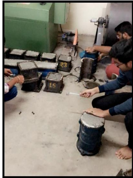
Figure 1. Demoulding the specimens
