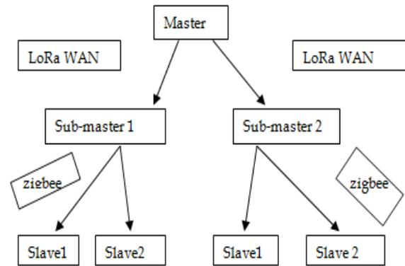
Figure 4 Master-slave network architecture
