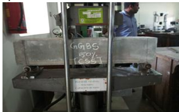
Fig.3 Flexural Strength Test prior to Crack
