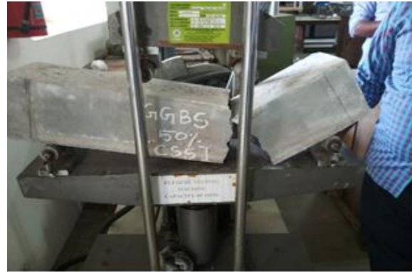
Fig.4 Flexural Strength Test at Crack
