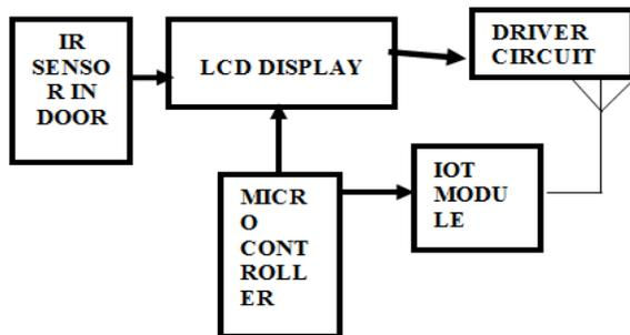
Fig. 1 Block Diagram of hardware Section
