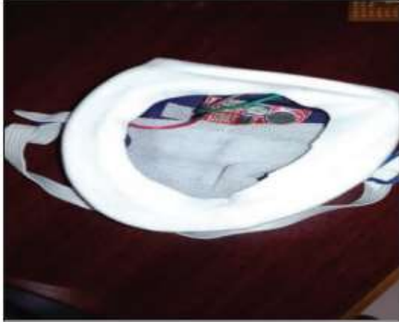
Fig. 6: Respiration Sensor with Face Mask
