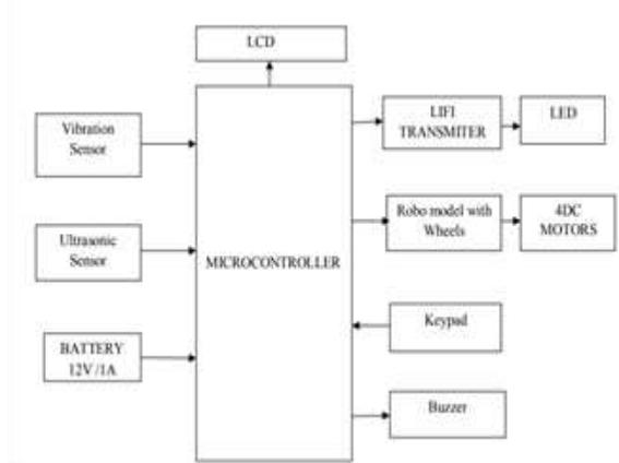
Fig 3: Transmitter Block Diagram
