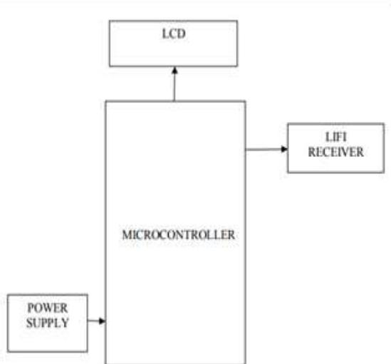
Fig 4: Receiver Block Diagram
