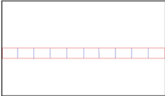
The count of white pixel in every unit in reference to black pixels is numbered respectively. This number determines the vehicle command.
