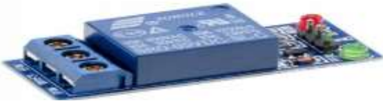
Figure8: relay with driving unit (module)
