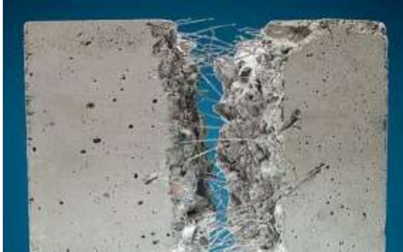
Fig. No. 1.1 Different Fiber in Concrete Cube after Tested
