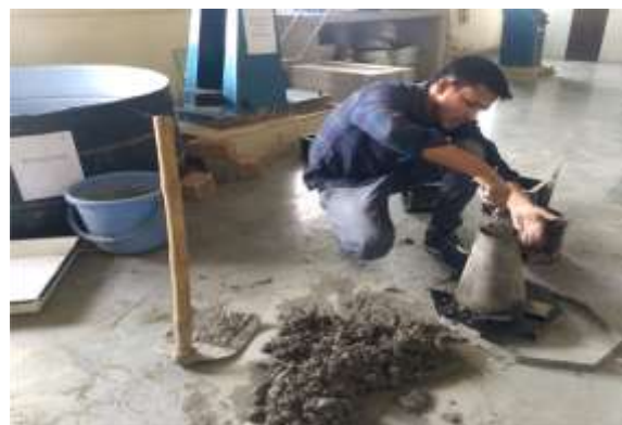
Figure 2.1 Concrete mixes for M-40 (Slump Cone Test of concrete)
