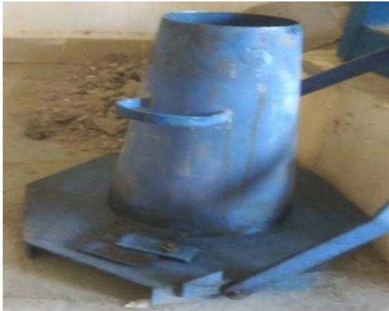
Fig. Slump cone testing
