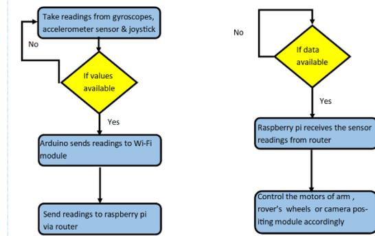
Fig.2,3 flow chart at operator and rover side
