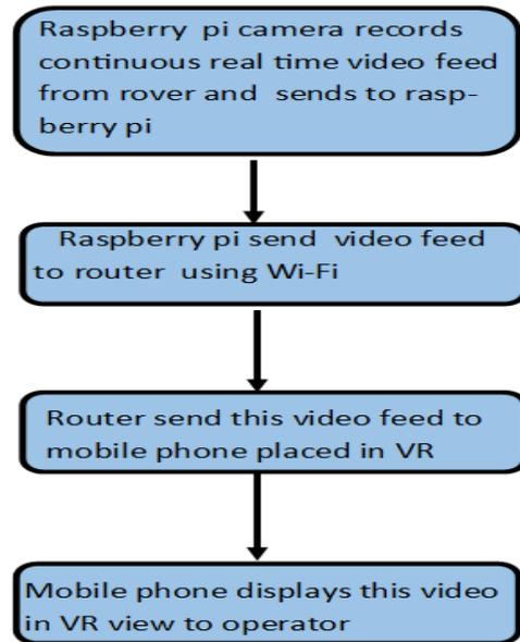
Fig.4 flow chart of operation of video streaming
