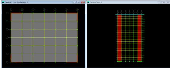
Fig.3 Model 2- shear wall at two corners of each wall
