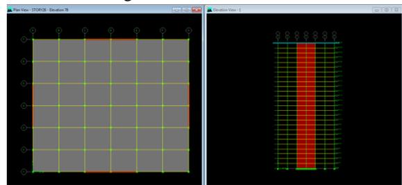
Fig.2 Model 1-shear wall at mid of outer walls
