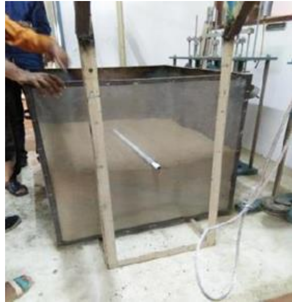
Fig. 4. Installation of nail
