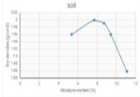
Figure 3.3 soil without reinforcement
