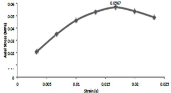
Figure 3.5 soil without reinforcement
