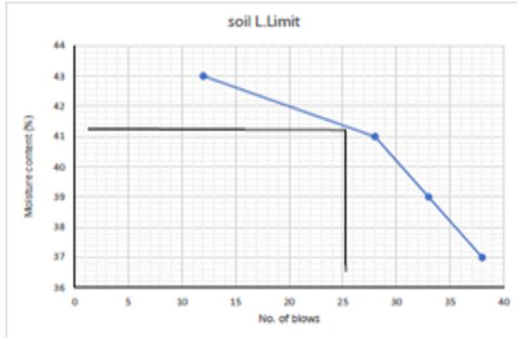
Figure 3.1 liquid limit for soil
