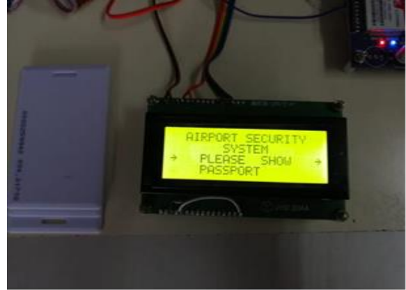
Figure 5 Requisition for passenger to swipe passport embedded with RFID tag
