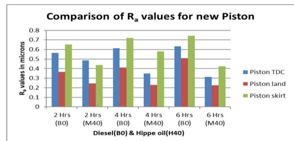
Figure 1 Comparison of Ra values for new piston (B0 and M40)
