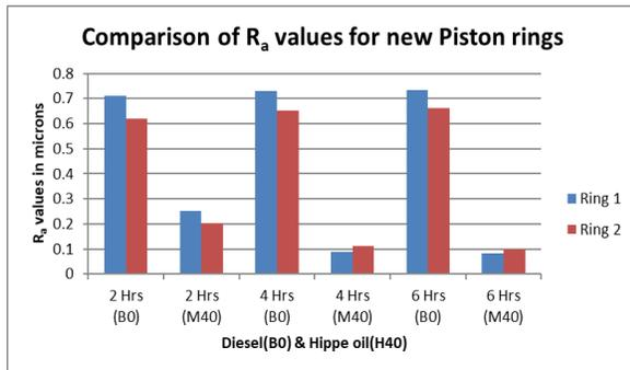
Figure 2 Comparison of Ra values for new piston rings (B0 and M40)
