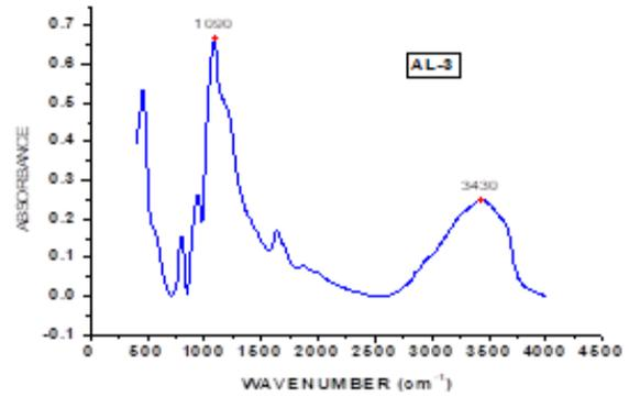
Fig. 2: The FTIR patterns of various concentrations of Er<sub>2</sub>O<sub>3</sub> Yb<sub>2</sub>O<sub>3</sub> silica gel
