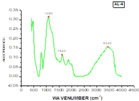
Fig. 3: The FTIR patterns of Er<sub>2</sub>O<sub>3</sub> Yb<sub>2</sub>O<sub>3</sub> silica gel
