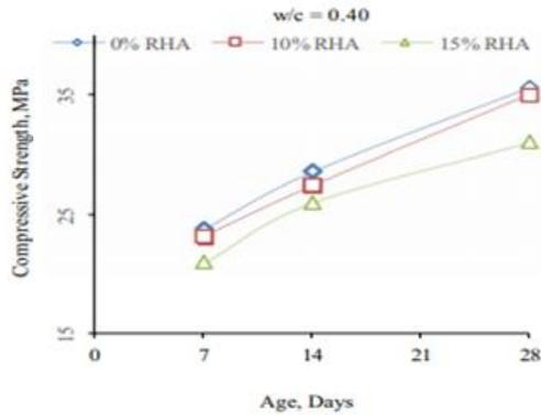
Graph 3 Compressive strength with w/c ratio 0.40
