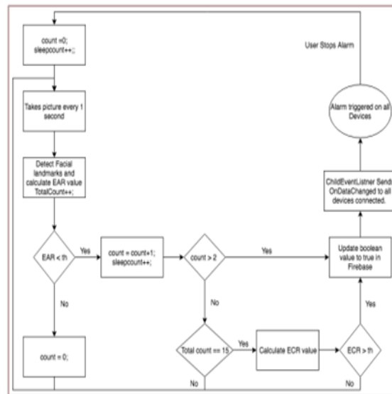
Fig. 2 - Block Diagram of Proposed Drowsiness Detection Algorithm
