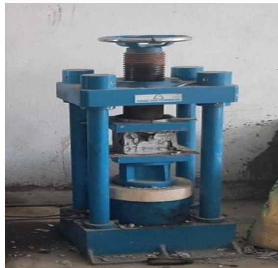
Figure 4: Arrangement & Failure of Specimen
