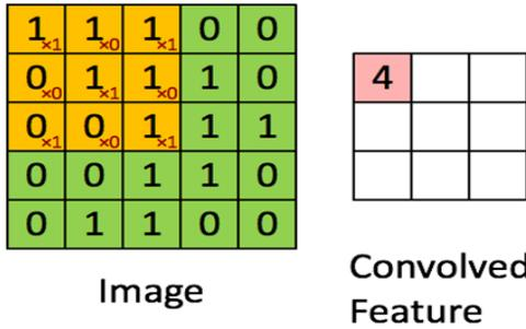
Convoluting a 5x5x1 image with a 3x3x1 kernel to get a 3x3x1 convolved feature
