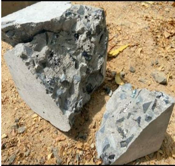
Figure-4 Failed Cube Specimen
