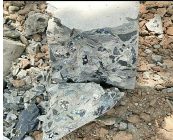
Figure-6 Slag in failed specimen
