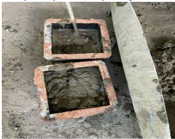
Figure-2 Concrete cubes while casting
