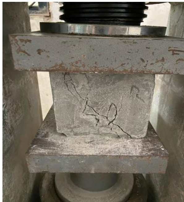
Figure-3 Concrete cubes while testing
