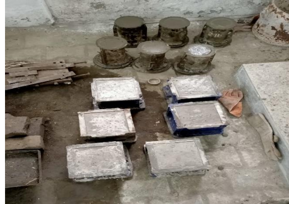
Fig 2. Samples for compression and split tensile strength test
