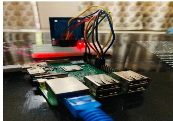
Fig. 4.6 Raspberry Pi and RFID Reader
